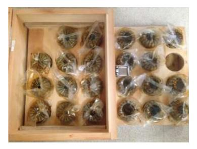
Set of 22 collets with a range from 4mm to 26mm.
